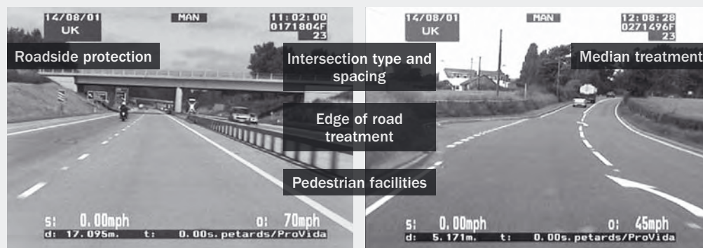
Figure 2 Similar high-level design elements can be assessed on roads of differing standard
